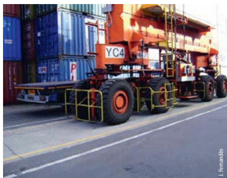
Photo 8 Détail essieux RTG Detail of RTG (gas turbine train) axles
