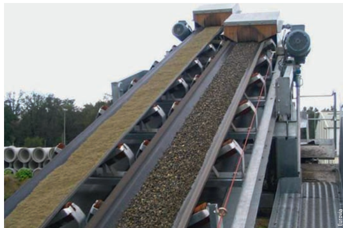
Photo 5 Poste d'enrobage à l'émulsion : des installations devenues performantes Emulsion based mixing plant: increasingly efficient installations
